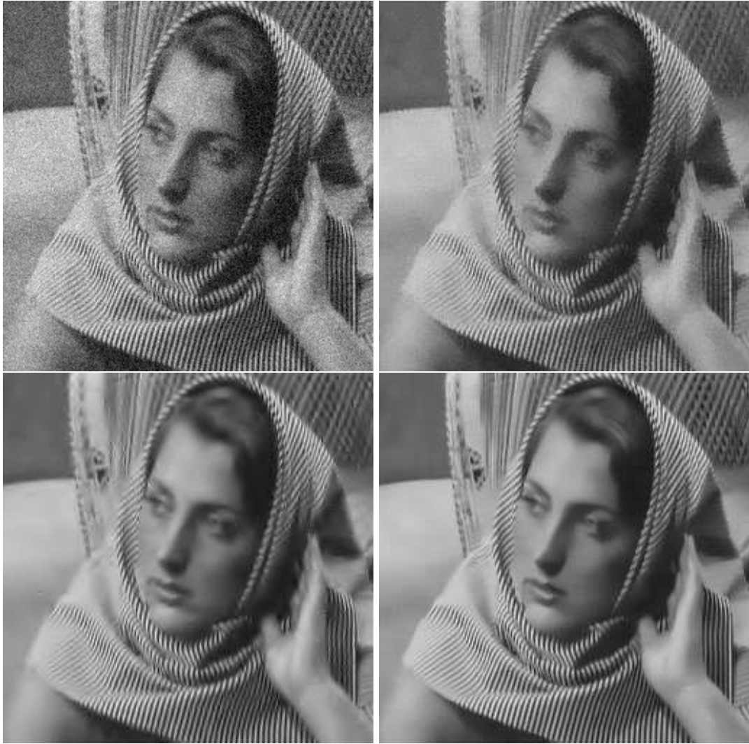
Figure 19: Comparison experiment. From top to bottom and left to right: noisy image, sigma or bilateral filter, translation invariant wavelet thresholding and the sliding window NL-means with the optimal linear correction. More image details are kept or even restored in the image denoised image by NL-means. However, a fully denoised image looks unnatural as all natural images have everywhere a microtexture similar to white noise, even if not due to captors. This is why industrial software add some white noise to restored images and movies. It is not the object of the present paper to discuss this esthetic aspect of image restoration.
